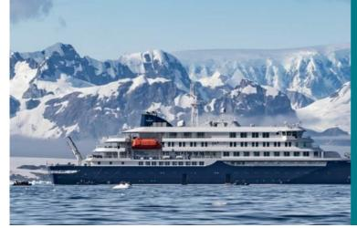
m/v Hondius Length : 107.6 meters Breadth : 17.6 meters Draft : 5.30 meters Ice class : Polar Class 6 (equivalent 1A-Super) Displacement : 5,590 tonnes Propulsion : 2 x ABC main engines; total 4,200 kW Speed : 15 knots Passengers : 170 in 80 cabins Staff & crew : Crew 57 | Guides 13 | Doctor 1
